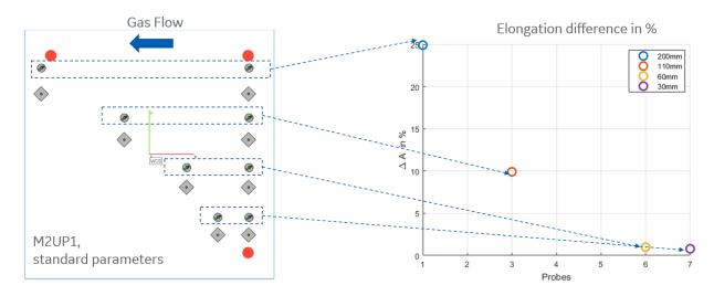
**Figure 3:** Sample build job to investigate laser-soot interaction regarding the mechanical properties of stainless-steel samples. Left: build plate set-up. Right: Elongation difference between reference sample on the right and corresponding sample on the left. Image credit: GE Additive
