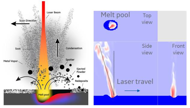
**Figure 1:** Conceptual depiction of interaction of powder, laser, and soot plume (left) and simulation results of showing temperature distribution (right). Image credit: GE Additive
