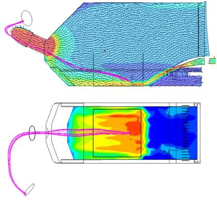
**Figure 6:** Streamlines of soot particles and velocity distributions in a Concept Laser M2 Series 4 machine flow environment. Top: side view, bottom: top view. Image credit: GE Additive
