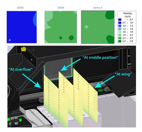
**Figure 5:** a) Evolution of build plate velocity from Gen 3 to Series 5 (left to right). A significant improvement of the flow field quality is observed.
