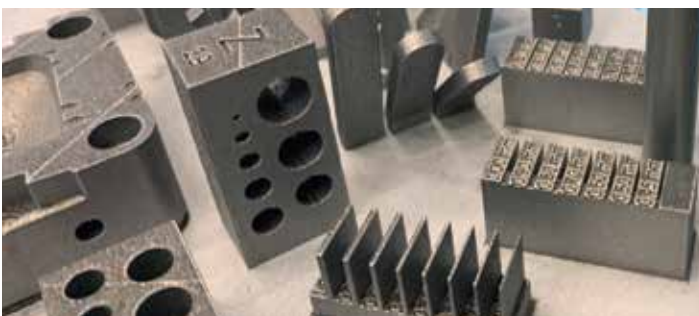
Printed fine features and gaps down to 200 \mu\text{m}
